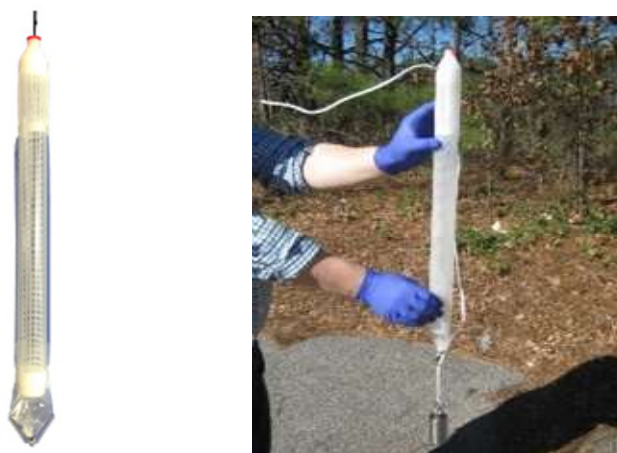
Figure 3: Dual Membrane Passive Diffusion Bag (DMDPB™) sampler. Provided by EON Products, Inc. under copyright. (Section 3.0)
