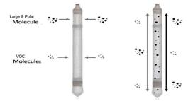
Molecules that enter the sampler through either membrane diffuse throughout the water inside of the sampler until dynamic equilibrium is reached within the sampler and with the surrounding groundwater. When the sampler is retrieved, water in the top membrane leaves the sampler through the large pores, while the lower chamber serves as a reservoir and retains the thoroughly diffused sample until discharged for analysis.
