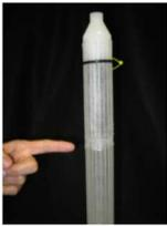
Until now, the reliable and economical use of passive diffusion sampling has been limited to non-polar VOCs because large or polar molecules and ions cannot pass through the polyethylene membrane into the sampler. EON's Dual-Membrane Passive Diffusion (DMPDB) sampler operates under *the same principles as the well established PDB sampling*, using two semi-permeable membranes in a single sampler, to capture an expanded list of compounds.
