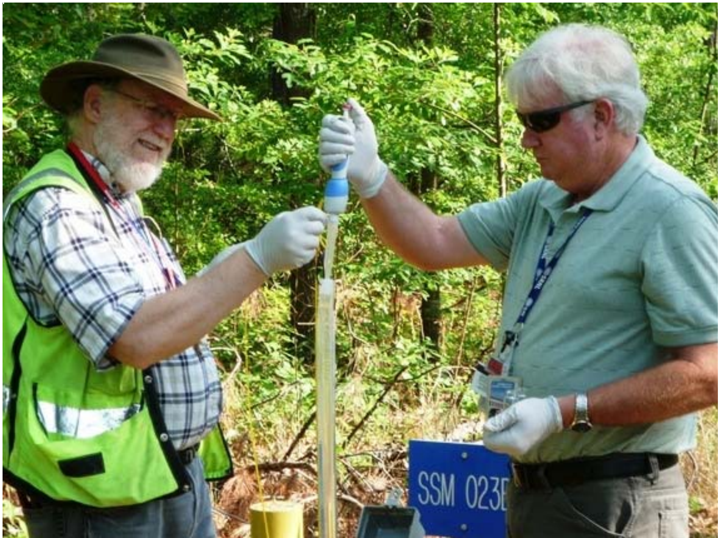
Savannah River National Laboratory Engineering Specialist Keith Hyde, right, and Savannah River Nuclear Solutions Geologist Bob Craig use a disposable Hydrasleeve sampler to monitor groundwater as part of efforts to meet regulatory requirements at the Savannah River Site.
