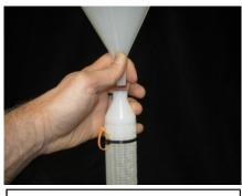
Place funnel inside the sampler nozzle. The extension tube (not shown) should be inserted into the sampler as far as possible.
