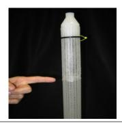
Pour De-Ionized water into sampler and fill to where the membranes meet. If the sampler is overfilled water will leak out of the upper membrane. *Seeping from the top membrane is normal if overfilled.* KEEP THE SAMPLER UPRIGHT !
