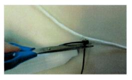
The Black Tie is attached to the sampler and has a "stop" on the other end. The tie is vertical (as shown) when the sampler is installed.
