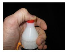
Place the Plug into the Nozzle and press firmly until the top of the plug rests against the Nozzle. . KEEP THE SAMPLER UPRIGHT !
