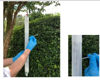
Note: **Do NOT** attempt to pour the sample from the top of the sampler as contents will leak out of the upper membrane while pouring.
