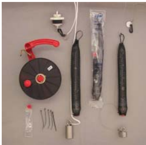
Figure 8-3. EON diffusion bag sampler and supplies
