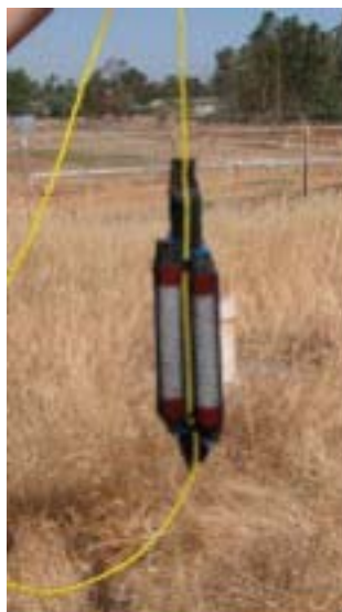
Figure 9-2. Two RPPSs attached side-by-side along other passive sampling devices on a deployment rope
