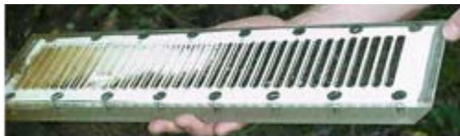
Figure 7-2. Box corer peeper sampler
