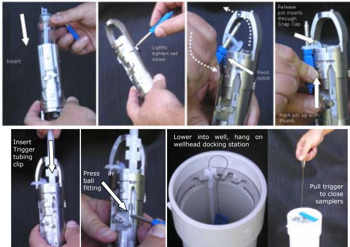
Figure 3-2. Snap Sampler™
