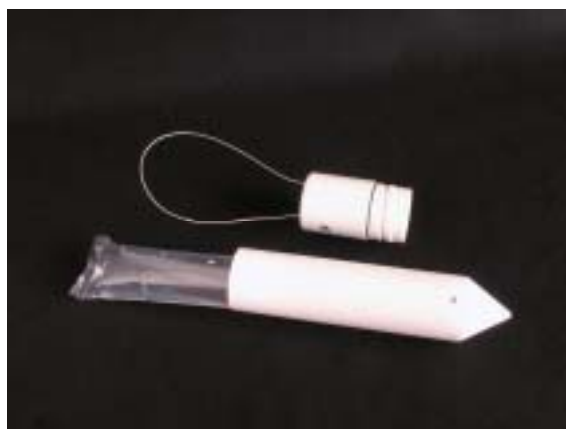
Figure 8-4. Protective screen canister for PDB deployment in sediments
