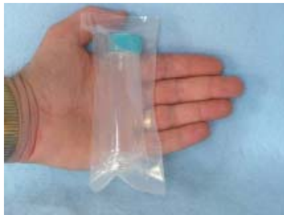
Figure 6-3. PVD to scale in hand (Photo from Church and others, 2002)
