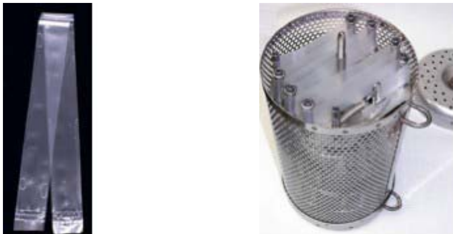
Figure 10-2. SPMD (left) and a surface water deployment canister containing 5 SPMDs (right). Deployment canisters are commercially available for groundwater monitoring wells as well.
