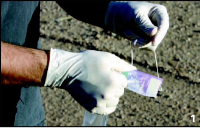
First, squeeze the full sampler just below the top to expel water resting above the flexible check valve. (Photo 1, top left)
