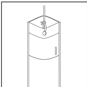
**3** Attach line to hole at top of HydraSleeve.
