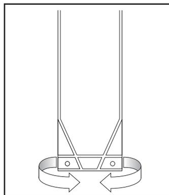
**4** Fold the two holes at bottom of HydraSleeve together and attach weight
