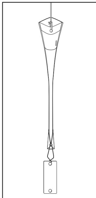
**5** Sampler is ready to insert into the well.
